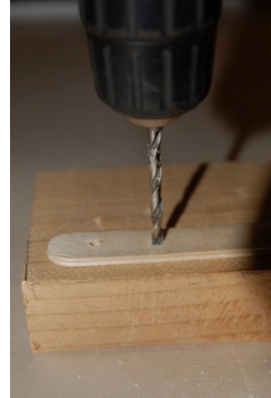
Drilling two holes through first and into second stick
